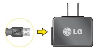
2. Plug the small end of the charger into the phone's Charger/Accessory Port and the other end into an electrical outlet.
