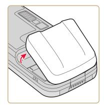
**4** Insert the bottom of a fully charged battery into the CS40, and press down firmly on the top of the battery. Make sure that the battery release tab is fully engaged (locked).
