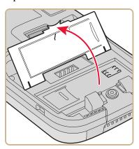
**4** Place the SIM card into the slot in the card access door.
