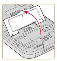
**4** Slide the microSD card door to the left to unlock it and open the door.
