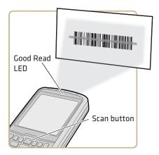
**5** Use the scanning beam as a guide and aim toward the middle of the bar code.
