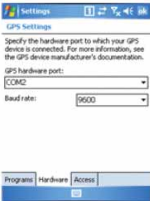
Set the Hardware port of the device. GPS hardware port for the M3 Mobile is COM2 and with baud rate of 9600.
