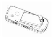
Finally refit the cabinet cover. It has to be put on the phone so that the cover lies on the phone without any gaps. Then - as the last step - press it down until it clicks into place.
