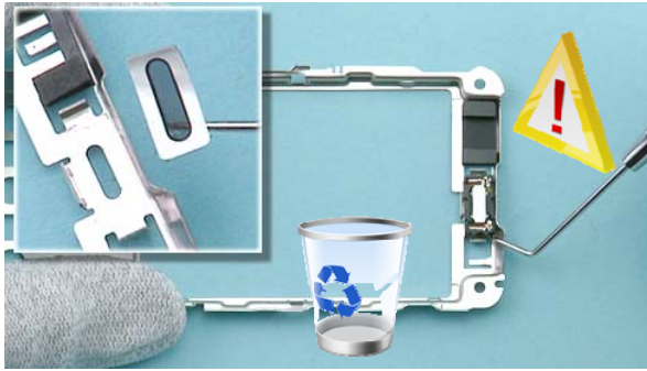
13) Detach the EARPIECE PIONEER and the EARPIECE NXP with the dental tool. Be aware of the sharp point of the dental tool!
