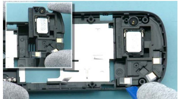
18) Use the SS-93 to lift up the ANTENNA MODULE from the D-COVER ASSY and then separate the module.
