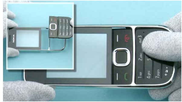
8) Separate the KEYMAT ASSY from the A-COVER by pressing the keymat lightly. When the keymat is separated protect both sides of the window with protective film to avoid scratches.
