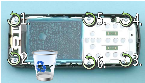
9) Unscrew the six TORX + size 6 screws in the order shown. Do not use it again.
