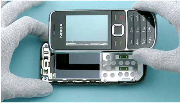
7) Remove the A-COVER ASSY. Make sure that the LCD is protected with protective film after removing the A-COVER ASSY.
