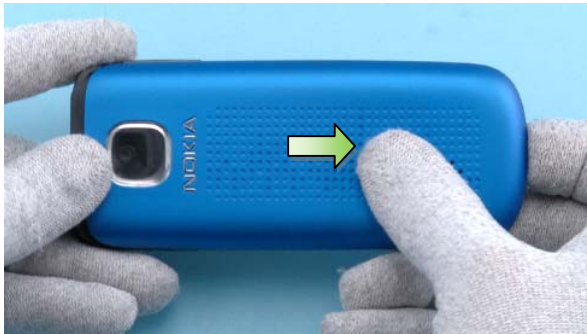
3) Slide the BATTERY COVER in the direction shown to release it.
