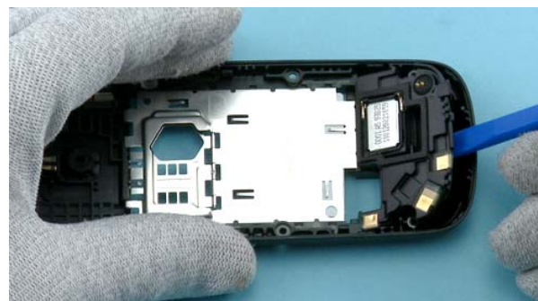
24) Use the SS-93 to lift up and separate the ANTENNA MODULE from the D-COVER ASSY.
