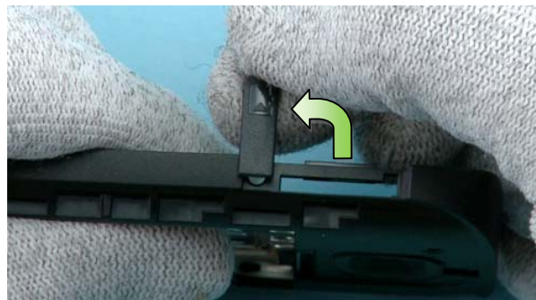
28) Open the SD COVER. Rotate and pull out the SD COVER through the small opening.
