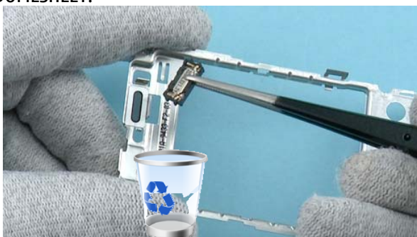
23) Remove the EARPIECE with the tweezers. Do not use it again. Discard it.
