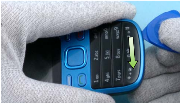
7) Then release the clips on the bottom side.
