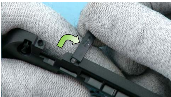
27) Rotate and pull out the USB COVER through the small opening.
