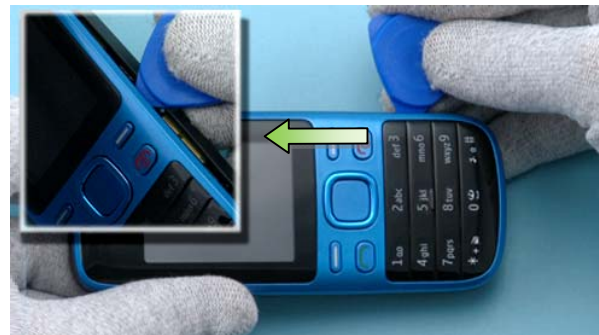
6) Slide the SRT-6 in the direction shown to release the clips of the A-COVER.
