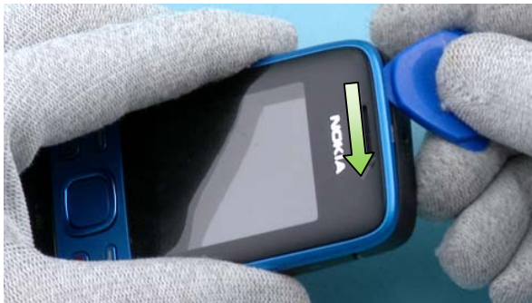
9) Slide the SRT-6 along the top side to release the remaining clips.
