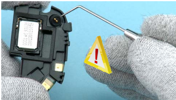
25) Use the dental tool to carefully lever out the MICROPHONE.
