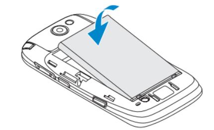
Align the battery's metal contacts with the connectors in the battery compartment and press the battery down until it locks into place.
