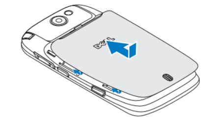
Insert the tabs on the back cover into the slots on the phone and slide the back cover into place.
