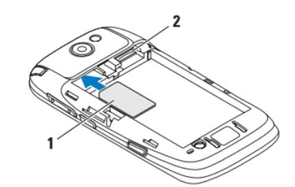
Slide the SIM card into the SIM card slot. Ensure that the SIM card's metal contacts are facing down and the beveled corner on the SIM card is facing the top of the phone.
