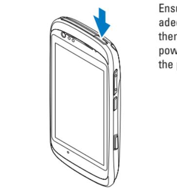
Ensure that the battery is adequately charged and then press and hold the power button to turn on the phone.
