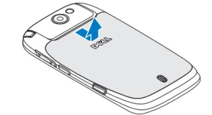
Press your thumb on the groove on the back cover and slide the back cover down.
