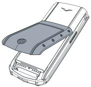
Pivot and slide the back cover into position until it clicks into place. The cover should close tightly using only light pressure – do not force it closed! If the cover does not close easily, remove it and check the battery is correctly inserted.
